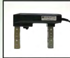
B300-MR Contour Probe is a rugged high performance instrument for magnetic particle inspection. This unit provides a strong AC field and includes Parker's original flexible leg design that allows the field to be "focused" at a precise area of inspection.
