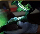
The B300-AR Contour Probe is a rugged high performance instrument for magnetic particle inspection. This unit provides a strong AC field and includes Parker's original feed-the-rod design that allows the field to be "focused" at a precise area of inspection.
