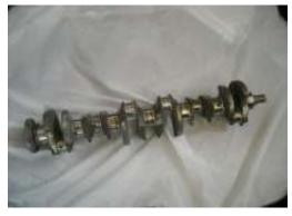
Std rod std main journal stroke 3.895. Rated at 800hp all new 5140 high-grade steel. .090 Radius micro polished and Zero balanced. Will fit all 4.0 and 258 Blocks call for pricing available March
