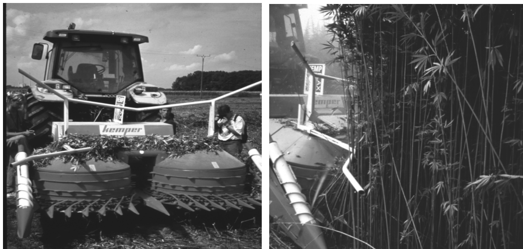
Figure 4. A modern European forage chopper (left) cutting and windrowing hemp (right) (Leson, 1996).
