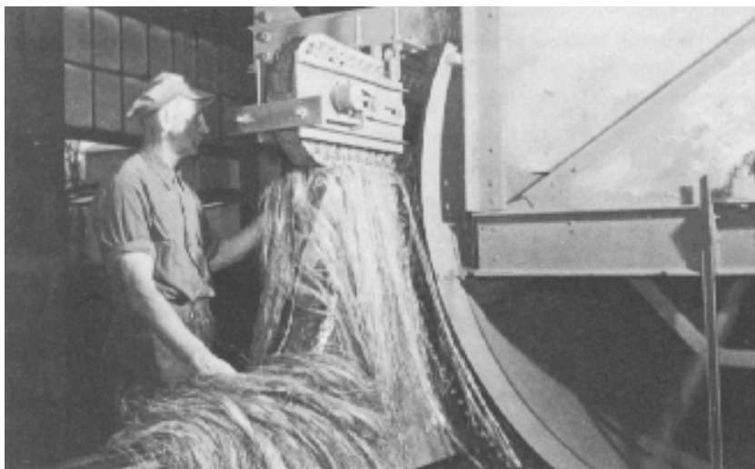
Figure 6. Hemp fiber emerging from the scutcher (Dempsey, 1975).
