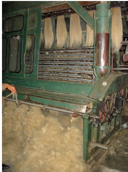
Combing machine separating the long hemp fibers (top) from the short hemp fibers (bottom).
