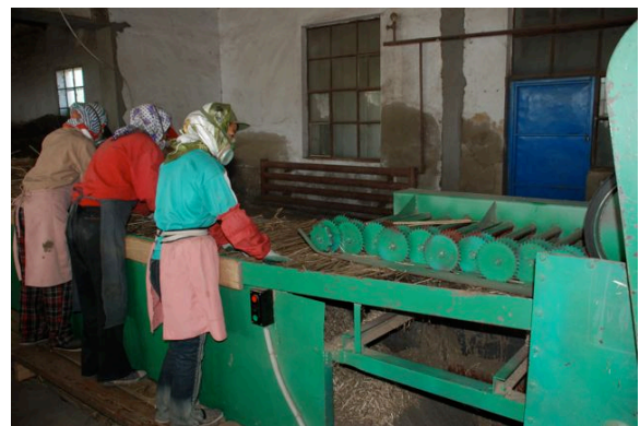
Hemp stalks pass under a series of rollers to break them down. The bast fiber is collected at the top while the huds are collected at the bottom
