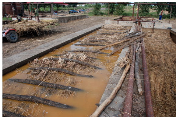
Tanks of water can be temperature controlled and the waste neutralized.
