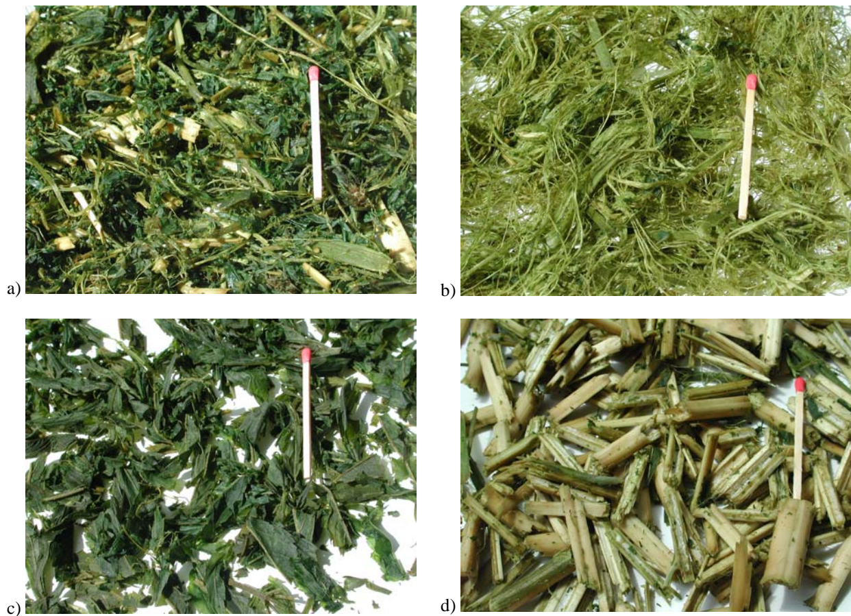
Fig. 4: Manually sorted, hand-chopped material: a) chopped material, b) fibres, c) leaves, d) shives
