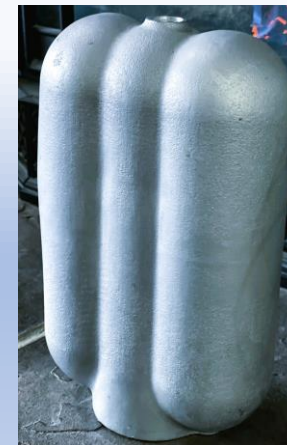
Actual casted Prototype of New Hydra Tank
