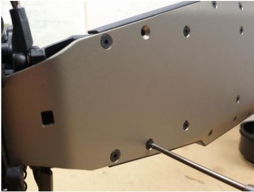
Remove the rearward factory screws from the servo mount. Replace them with the 18mm stainless steel screws supplied in the mid mount kit.
