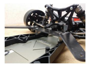
Attach the mid mount to the stand offs using the supplied 6mm button head screws. Attach the body posts to the mid mount.
