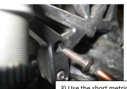
2) Reuse the longer factory bumper mounting screws to bolt on the mod bumper. The factory screws will be inserted into the rear most mounting holes on the mod bumper. The long metric screws provided with the kit will then be inserted into the forward most mount holes in the bumper.
