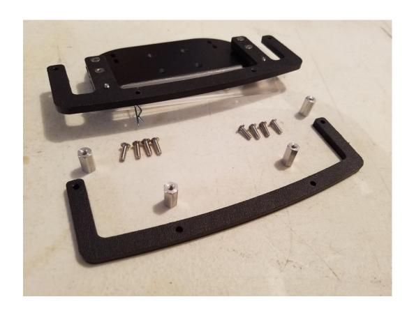
ATTACH THE UPPER "TUBE" BUMPER SECTION TO THE LOWER "TUBE" BUMPER SECTION USING THE (8) SUPPLIED 3/8' BUTTON HEAD SCREWS AND (4) SUPPLIED 1/2" LONG STAND OFFS.
