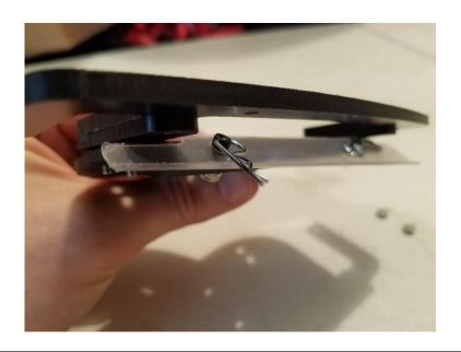
ATTACH THE LOWER "TUBE" BUMPER SECTION TO THE BUMPER PLATE USING THE 4 SUPPLIED 5/8" FLAT HEAD SCREWS AND LOCK NUTS. NOTE THAT THE SUPPORT BRACKETS ARE SANDWICHED BETWEEN THE "TUBE" BUMPER AND THE BUMPER PLATE.
