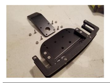
ATTACH THE BUMPER PLATE ASSEMBLY TO THE BUMPER PLATE MOUNT USING THE (4) SUPPLIED  $\frac{1}{2}$ " FLAT HEAD SCREWS AND LOCK NUTS.
