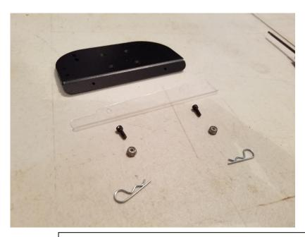
ATTACH THE SPLITTER TO THE BUMPER PLATE USING THE SUPPLIED CROSS DRILLED BUCKET HEAD CAP SCREWS AND LOCK NUTS. THE BODY CLIPS WILL BE USED LATER TO SECURE THE NOSE PANEL TO THE BUMPER PLATE.
