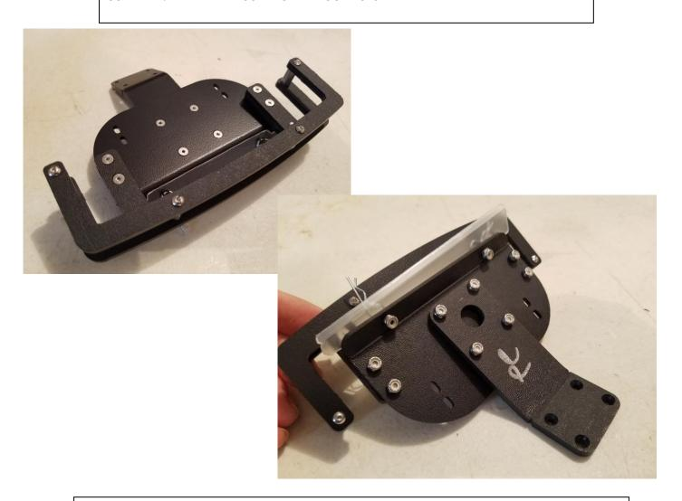
IN MOST BUMPER KITS YOU WILL FIND A BUMPER PLATE SUPPORT BRACE. THIS PIECE USUALLY BOLTS TO THE FRONT SHOCK TOWER AND THEN DOWN TO THE BUMPER PLATE. THEY ARE CHASSIS SPECIFIC AND PICS CAN BE FOUND IN THE MOUNTING KIT INSTRUCTIONS.
