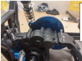
Remove the factory button head screws and replace with the supplied threaded rods. The  $\frac{1}{2}$ " long rods go in the most forward holes in the gearbox. The  $\frac{5}{8}$ " long rods go in the rearward most holes.
