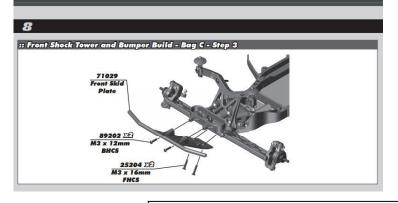
Attach the modified bumper plate to the chassis using the factory hardware. Attach the bumper support to the bumper plate and front shock tower using the supplied hardware.
