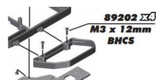
Remove the factory screws holding the nerf bars to the chassis. Attach the mid body post mounts to the nerf bars using the supplied hardware.
