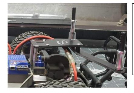
Attach the rear body mount to the stand offs using the (2) 3/8" long flat head screws.
