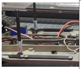
Remove the screws holding the nerf bar to the chassis.
