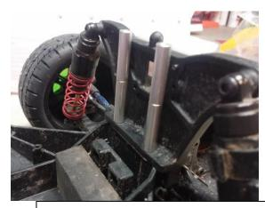
Remove the 2 screws that hold the front of the rear shock tower to the chassis.
