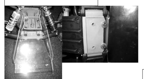
Attach the modified bumper mounting bracket to the underside of the front bulkhead using the (4) factory screws.
