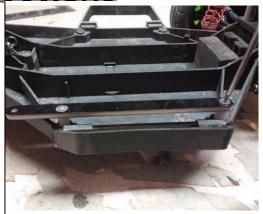
Remove factory front body mount, factory front bumper and factory from bumper support. Keep all hardware as it will be needed to mount the mod bumper and support to the front bulkhead.
