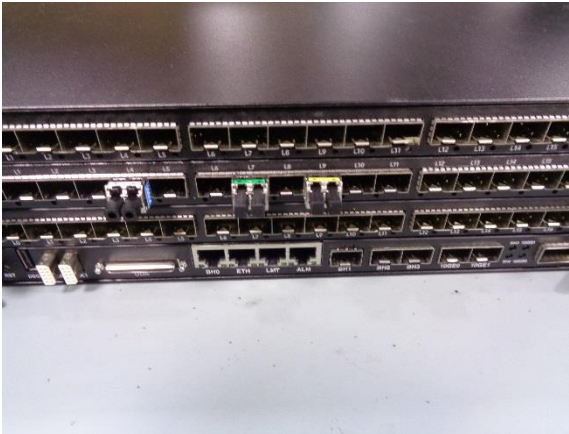
1. Optic module installation in CDU
