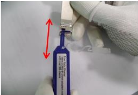
Push & pull the cleaner 2 to 3 times to remove the dust
