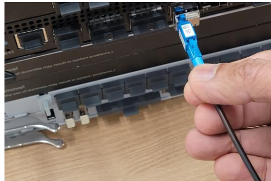
4. Select proper optic attenuator to make the measured power within normal RX power range
