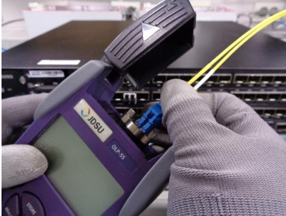
3. Measurement of optic power using optic power meter for "A" Port of optic cable in DU side
