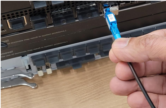
2. Optic attenuator must be Installed in CDU optic module before connection of optic cable
