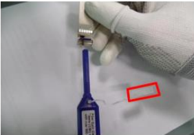
Remove the Cleaner "Guide Cap", Insert the Cleaner into TxRx port
