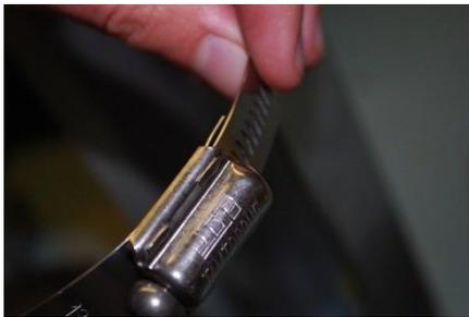
Push the end underneath the tamtorque mechanism as shown on the left
