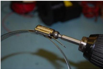
While pushing the fixing in this position, pick up the drill with the tamtorque bit and screw clockwise into the hole as shown on the left. This should then start to tighten around the post.
