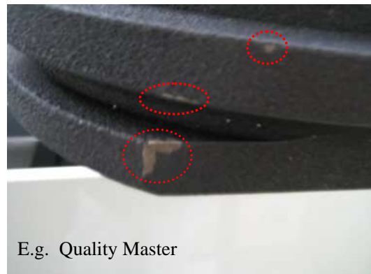
Coating peeling off of cast iron portion of main body
