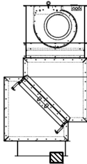
Once the adapter is secured to the machine, caulk the seam and fasten the unit to the adapter using the 12 bolt pattern on the bottom of the unit with 1/4" -20 bolts
