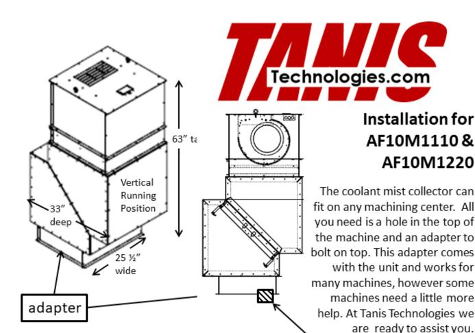
Once the adapter is secured to the machine, caulk the seam and fasten the unit to the adapter using the 12 bolt pattern on the bottom of the unit with ½ -20 bolts
