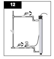
Open water supply to the UV system, and then close downstream tap.
