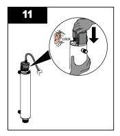
Push the lamp connector against lamp connector base together until an audible click is heard.
