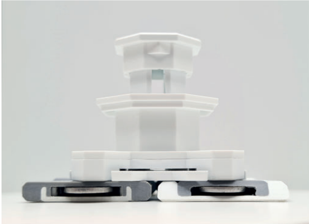
Lifter with revealed Accoustic Feedback Disks.
