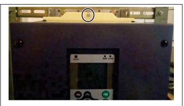
(2) Remove the two screws from the top of the fan casing.
