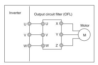
Figure 4.7 External View of Output Circuit Filter (OFL) and Connection Example
