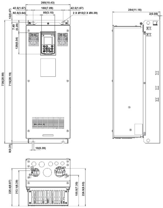
Figure 4 External Dimensions of the Inverter
