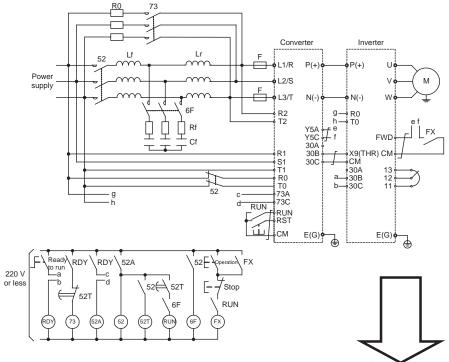
Connection diagram of replacement inverters (after replacement)
