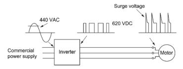
Figure B.1 Voltage Waveform of Individual Portions
