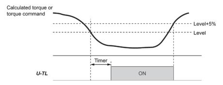
In the inverter's low frequency operation, as a substantial error in torque calculation occurs, no low torque can be detected within the operation range at less than 20% of the base frequency (F04). (In this case, the result of recognition before entering this operation range is retained.)
