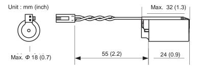
Figure 4.13 External View and Dimensions O
