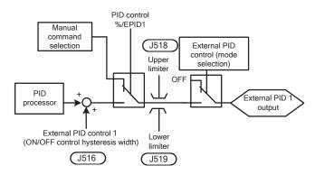
Also, by disabling I (integral time) and D (differential time) to enable only P (gain) and this value, the following comparison is possible.
