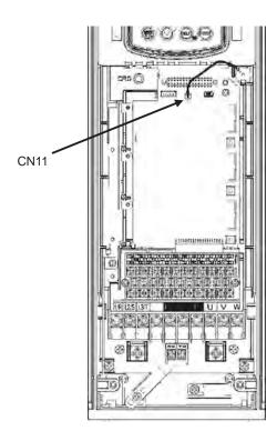
Figure 4.14 Battery Loaded (FRN005AR1■-2U or below, FRN010AR1■-4U/5U or below.)
