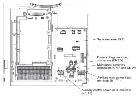
Figure 5.4-1 Location of Switching Connectors (230 V class series inverters of 30 to 60 HP and 460 V ones of 60 to 125 HP)
