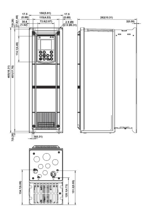
Figure 1 External Dimensions of the Inverter
