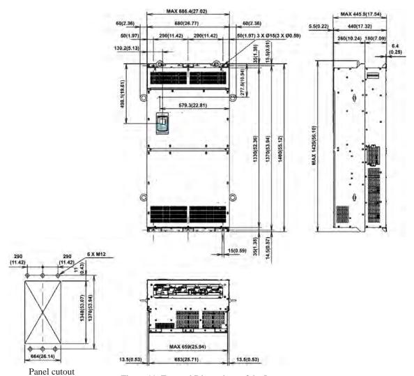
Figure 11 External Dimensions of the Inverter
