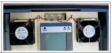
(2) Pull the latches securing the fans in the direction of the arrows and remove the fans.
