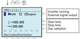
5. Use the ⟨⟨⟩ / ⟨⟩ keys to shift the cursor, and use the ⟨⟨⟩ / ⟨⟩ keys to input the check mark, time and day.
