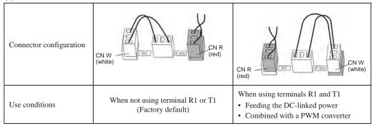
Note By factory default, the CN R is set on the 73X position (230 V class series inverters of 30 to 60 HP and 460 V ones of 60 to 125 HP) or on the FAN position (230 V class series inverters of 75 HP or above and 460 V ones of 150 HP or above), and the CN W is set on the NC position. Do not exchange them unless you drive the inverter with a DC-linked power
