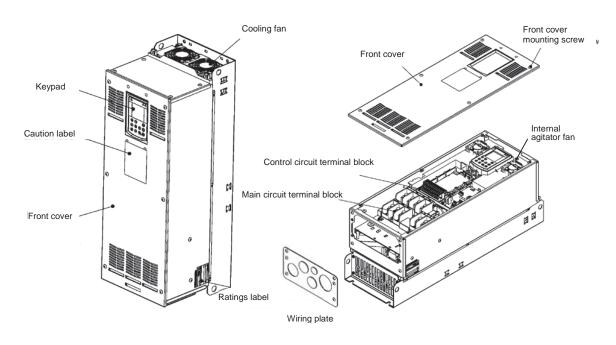
Fig. 1.6 FRN030-040AR1M-2U / FRN060-075AR1M-4U/5U ( NEMA/UL type 1)
