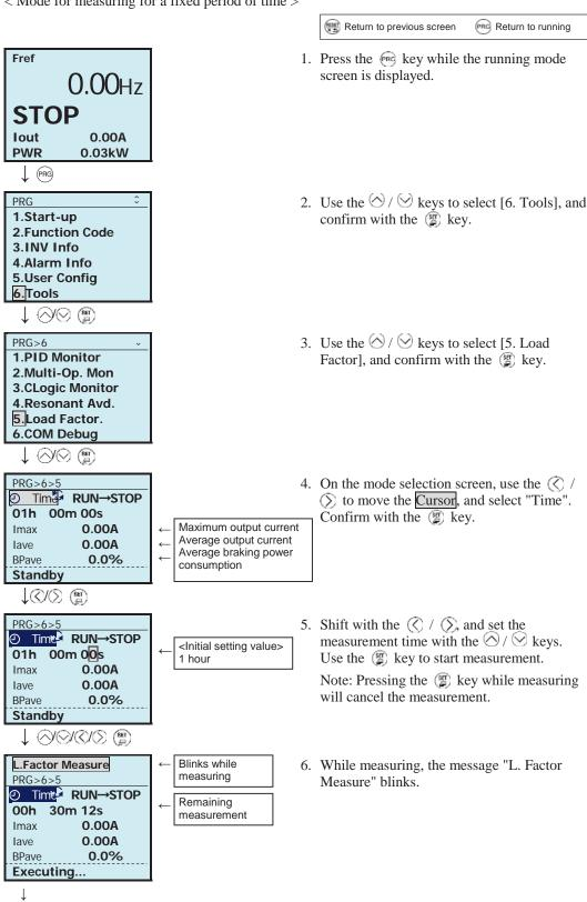
7. Measurement is concluded after the measurement time elapses, and measurement results are displayed.
