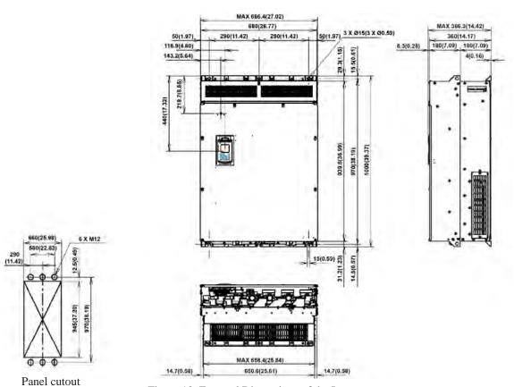
Figure 10 External Dimensions of the Inverter
