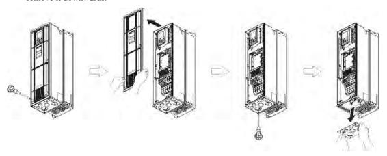
Figure 5.2 Removing the Front Cover and the Wiring Plate (FRN050AR1M-4U)
