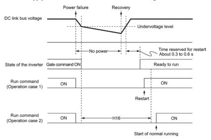
If H16 (Allowable momentary power failure time) is set to "Auto," restart will take place until the DC link bus voltage drops down to the allowable voltage (100 V) for restart after a momentary power failure. If the DC link bus voltage drops below the allowable voltage, the inverter recognizes that the power has been shut down so that the inverter does not apply the restart mode and starts normal running.
