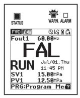
Fig. 9.1 Light alarm display example
