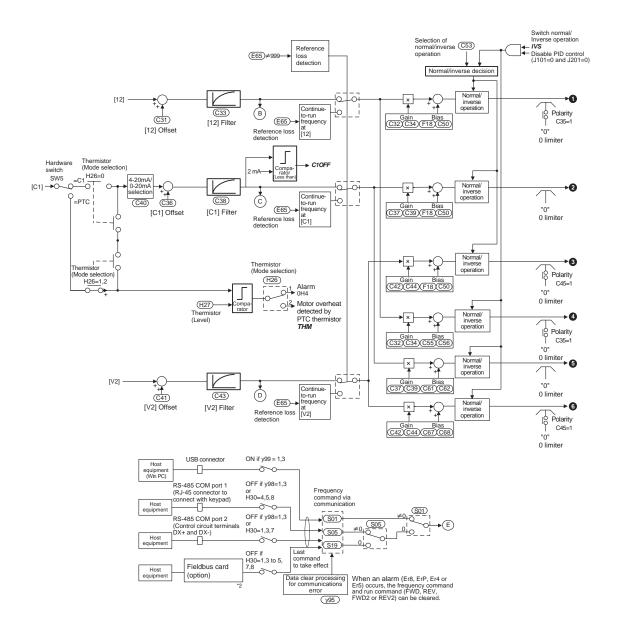
Figure 7.1 (1) Frequency Command Block
