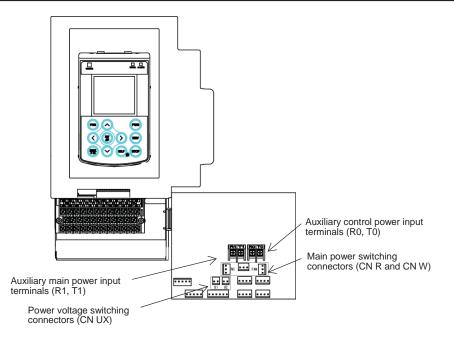
Figure 5.4-3 Location of Switching Connectors (460 V class series inverters of 250 HP or above)
