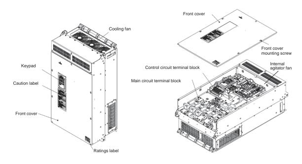
Fig. 1.9 FRN075-125R1S-2U / FRN150-1000AR1M-4U/ FRN200-300AR1M-5U (UL open type)
