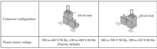
Note The allowable power input voltage fluctuation is within -15% to +10% of the power source voltage.
