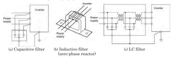
Figure A.10 Various Filters and their Connection
