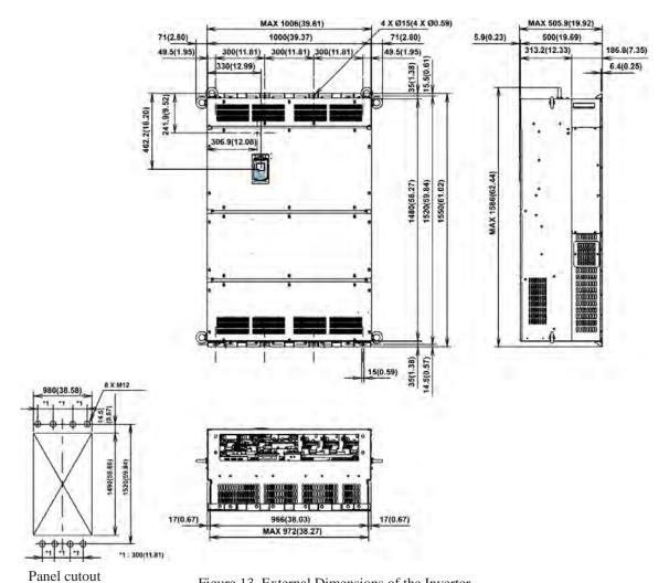
Figure 13 External Dimensions of the Inverter
