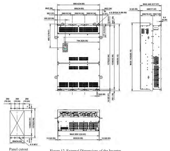
Figure 12 External Dimensions of the Inverter
