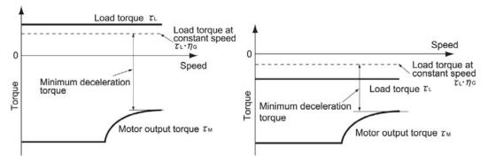
Figure 3.5 Example Study of Minimum Deceleration Torque (1)
