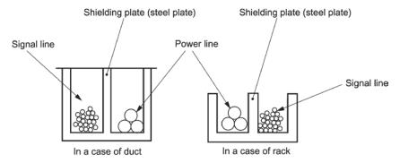
Figure A.7 Separate Wiring
