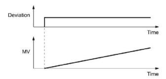
■ D differential time (PID control 1: J112 / PID control 2: J212)
