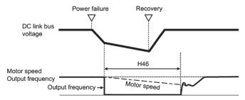
Under auto search control, the inverter searches the motor speed with the voltage applied at the motor start and the current flowing in the motor, based on the model built with the motor parameters. Therefore, the search is greatly influenced by the residual voltage in the motor.
