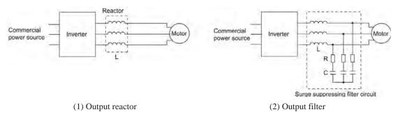
Figure B.3 Method to Suppress Surge Voltage
