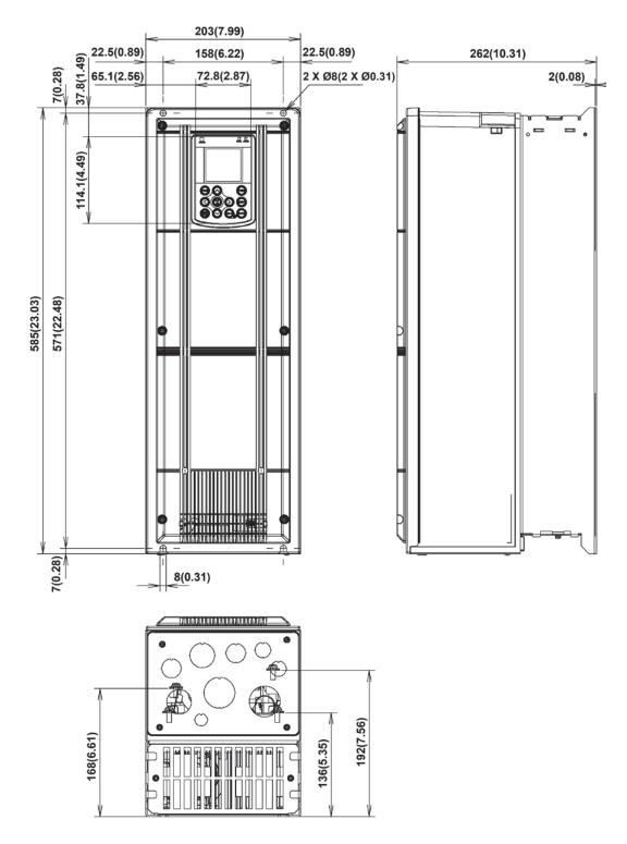
Figure 2 External Dimensions of the Inverter
