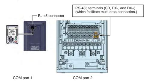
Using the RS-485 communications ports shown above enables the extended functions listed below.
