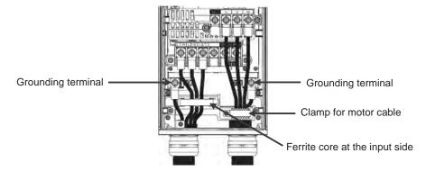
Figure 11.1 Wiring to Main Circuit Terminals for FRN020AR1∎-2U, FRN025AR1∎-2U, FRN040AR1∎-4U, and FRN050AR1∎-4U.
