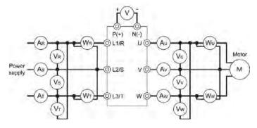
Figure 10.1 Connection of Meters
