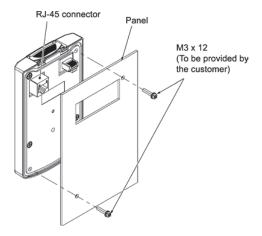
Figure 5.9 Mounting the Keypad
