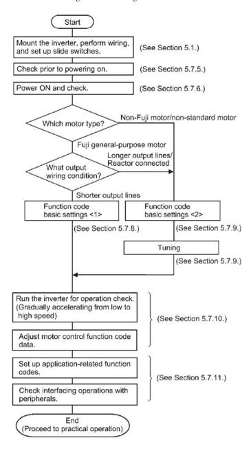
Figure 5.16 Test Run Procedure
