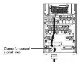
Figure 11.2 Wiring to Control Circuit Terminals for FRN020AR1∎-2U, FRN025AR1∎-2U, FRN040AR1∎-4U, and FRN050AR1∎-4U.
