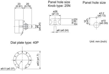
Note: The dial plate and knob must be ordered as separated items. Available from Fuji Electric Technica Co., Ltd.
