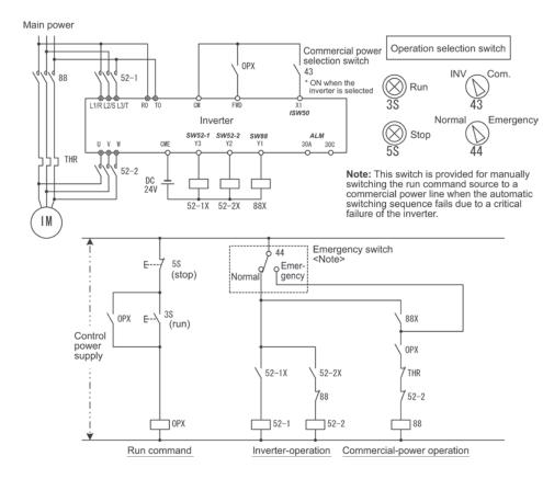
3) Sequence with an emergency switching function --Part 2 (Automatic switching by the alarm output issued by the inverter)
