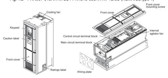
Fig. 1.3 FRN007-015AR1L-2U / FRN015-030AR1L-4U/5U (NEMA/UL type 12)
