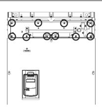
(4) The figure given at the right shows the removed fan unit. Fan unit (5) Cut off the cable ties (InsuLock) securing the Internal fan mounting plate internal fan cables. Internal fans AIR FLOW Remove the internal fan mounting screws and take the internal fans off the internal fan mounting plate. Cable ties (InsuLock) Internal fan mounting screws Internal fan cables (6) For inverters of 300 to 450 and 800 HP: Disconnect the terminals from the fan capacitors. Fan capacitors
