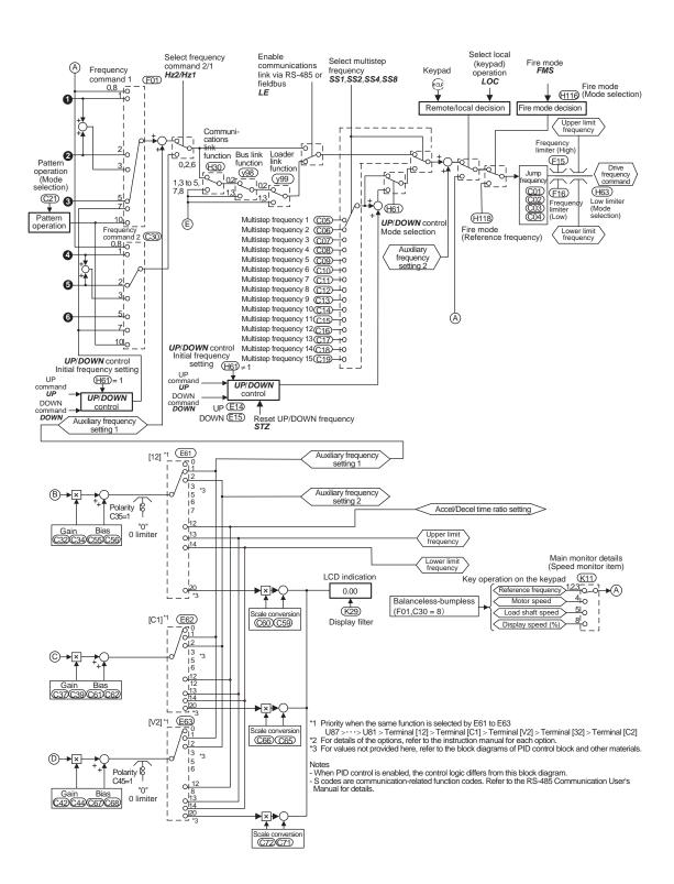
Figure 7.1 (2) Frequency Command Block
