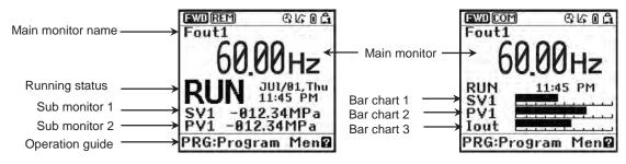
The display type can be selected easily in Programming mode as follows.
