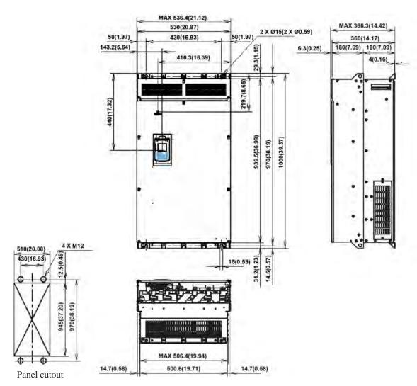
Figure 9 External Dimensions of the Inverter
