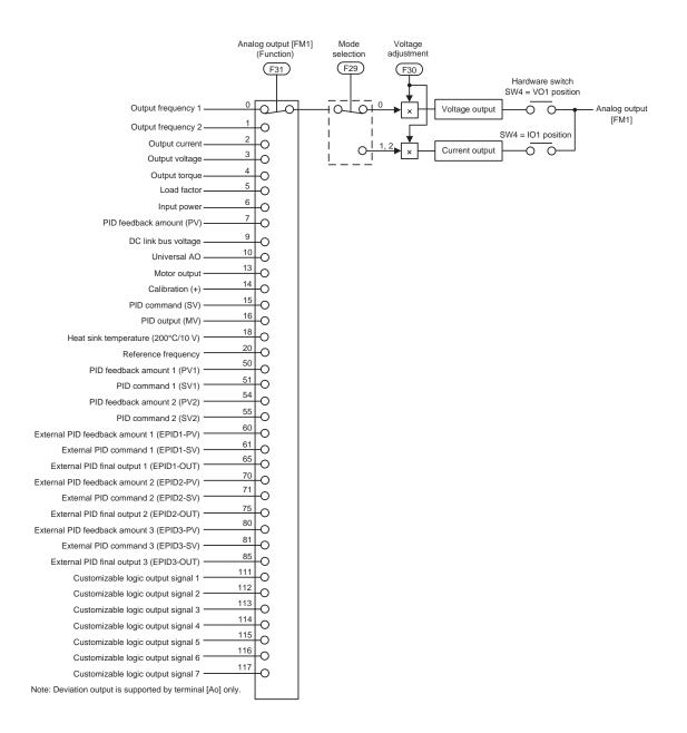
Figure 7.6 Terminal [FM1] Output Selector
