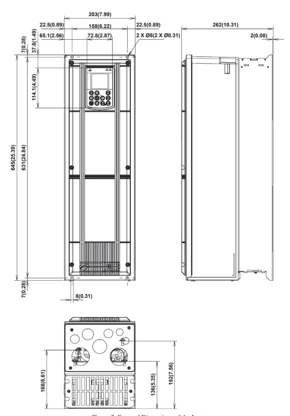
Figure 3 External Dimensions of the Inverter
