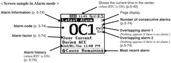
Figure 5.12 Screen Samples In Running and Alarm Modes
