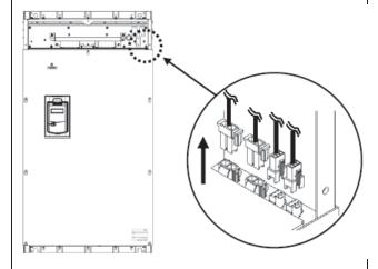
(3) Remove the fan unit mounting screws and pull out the fan unit towards you.
