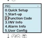
Use the ⟨○ / ⟨○ keys to select [2. Function Code], and confirm with the (② key.
