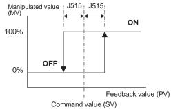
External PID Control 1 (Proportional operation output convergent value)
