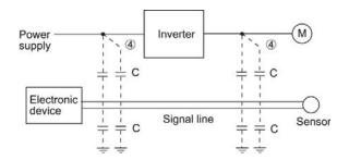
Figure A.5 Electrostatic Induced Noise
