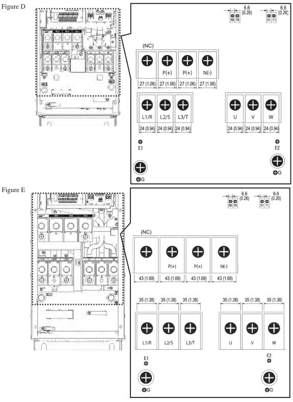
Unit: mm (inch) (NC): No connection (Do not make wiring.)
