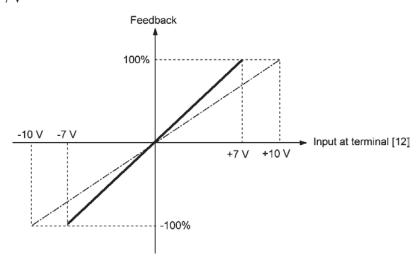
(Example 2) When the output level of the external sensor is 0 to 10 VDC:
