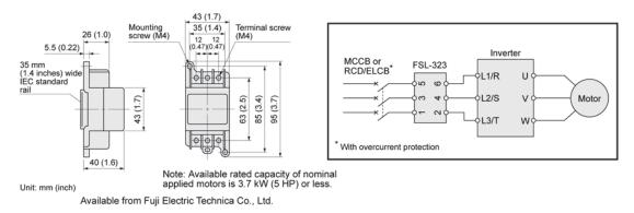
Figure 4.3 Dimensions of Surge Killer and Connection Example
