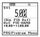
Figure 5.15 Setting the PID Process Command (display sample)
