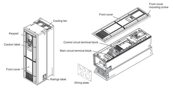
Fig. 1.4 FRN020-025AR1M-2U / FRN040-050AR1M-4U/5U (NEMA/UL type 1)
