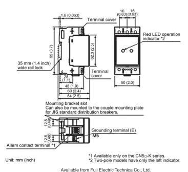
Figure 4.4 Arrester Dimensions and Connection Examples
