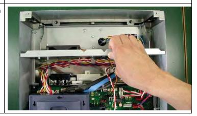
(4) The photo given at the right shows the fan unit removed.
