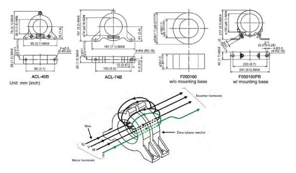
Figure 4.4-1 Dimensions of Zero-phase Reactor for Reducing Radio Noise (ACL) and Connection Example
