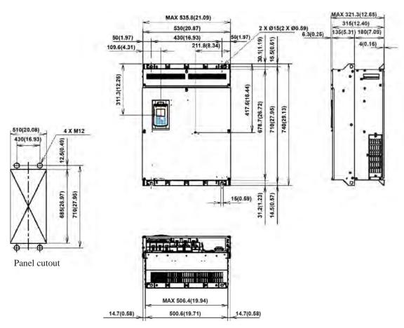
Figure 8 External Dimensions of the Inverter
