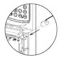
(3) Hook the battery harness over the boss and then fully insert the connector into connector CN11 on the control printed circuit board.
