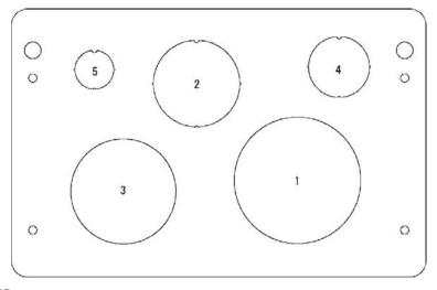
For instructions on how to punch out semi-perforated sections in the wiring plate and set conduits on the wiring plate, refer to Chapter 5, Section 5.1.2.1 "(2) Punching out semi-perforated sections in the wiring plate and setting cable glands or conduits."
