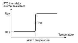
Suppose that the internal resistance of the PTC thermistor at the alarm temperature is Rp, the detection level (voltage)  $V_{\nu 2}$  is calculated by the expression below. Set the result  $V_{\nu 2}$  to function code H27.
