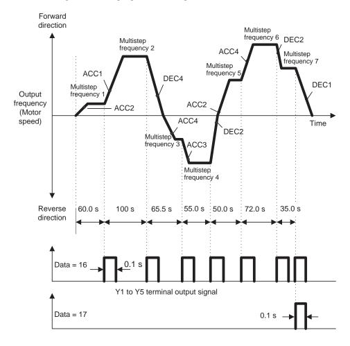
To start or stop a pattern operation, use the  $\widehat{\text{Fwo}}$  /  $\widehat{\text{Frop}}$  keys on the keypad or turn the related input terminals ON/OFF.
