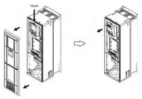
Figure 5.7 Removing the Keypad
