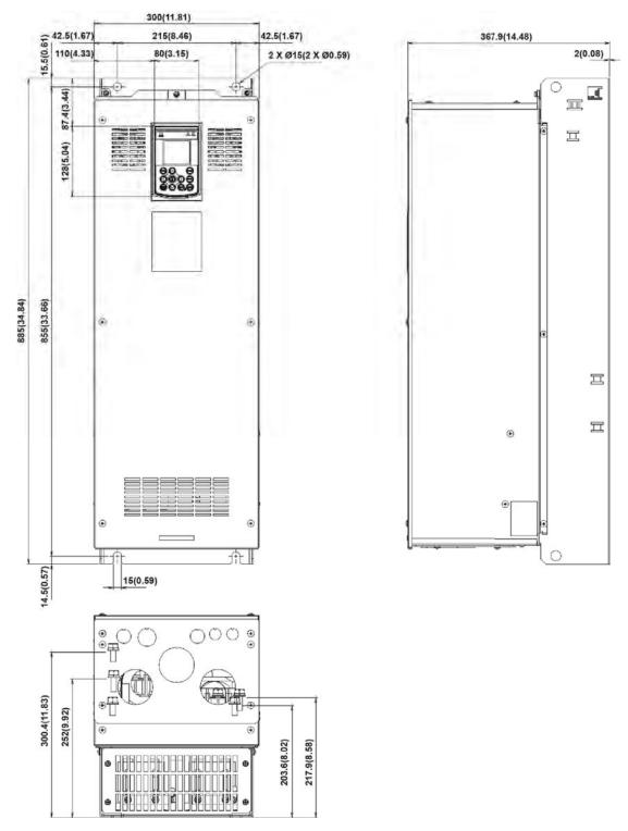
Figure 5 External Dimensions of the Inverter
