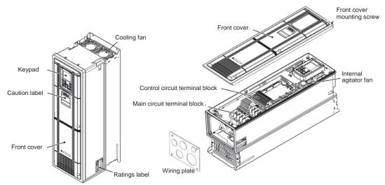
Fig. 1.5 FRN020-025AR1L-2U / FRN040-050AR1L-4U/5U (NEMA/UL type 12)
