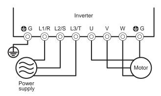
Figure 5.17 Connection of Main Circuit Terminals
