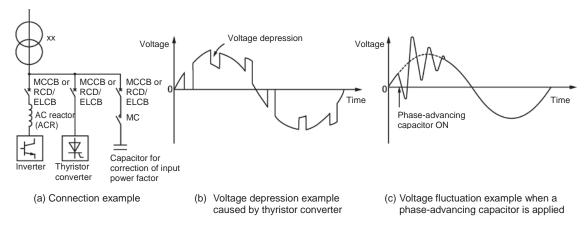
• Use an ACR when the interphase voltage unbalance ratio of the inverter power supply exceeds 2%.
