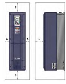
Figure 5.1 Mounting Direction and Required Clearances
