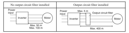
For an inverter with an output circuit filter installed, the total secondary wiring length should be 400 m (1312 ft) or less.
