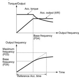
The figures at left show the acceleration characteristics. Similar characteristics apply to the deceleration.
