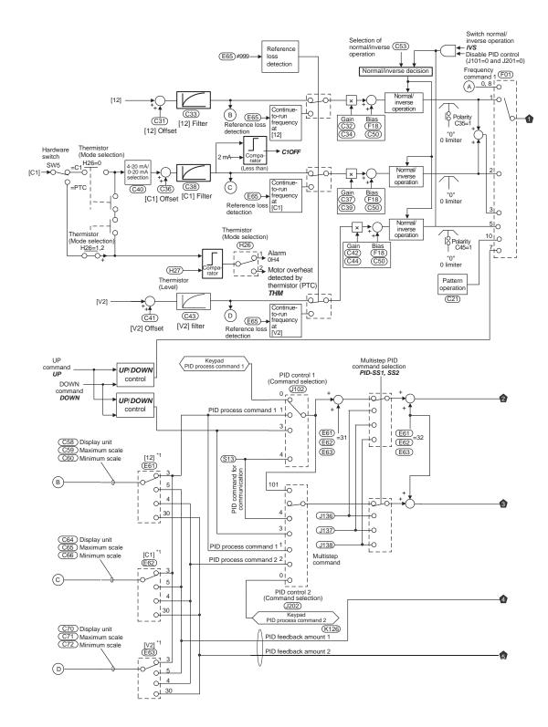
Figure 7.4 (1) PID Process Control Block
