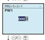
4. Use the ⊘ / ⊗ keys to input the password that has been set, and confirm with the ⟨𝔻⟩ key.
