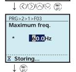
7. "Storing" is displayed, and data is saved to the inverter's internal memory.
