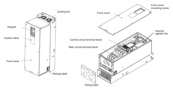
Fig. 1.8 FRN050-060AR1L-2U / FRN100-125AR1L-4U/ FRN100-150AR1L-5U ( NEMA/UL type 12)
