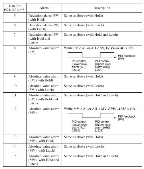
SV: Process command value, PV: Feedback value, MV: Manipulated value
