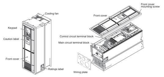
Fig. 1.2 FRN007-015AR1M-2U / FRN015-030AR1M-4U/5U (NEMA/UL type 1)
