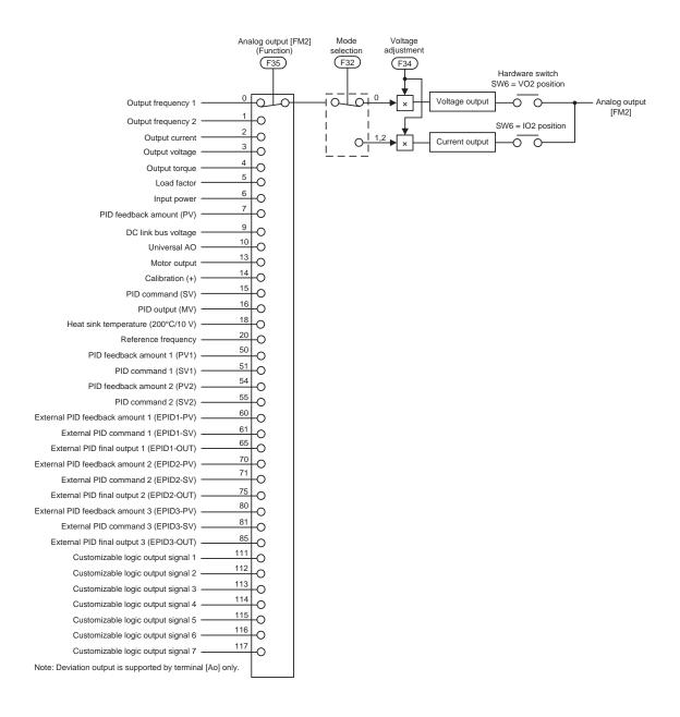
Figure 7.7 Terminal [FM2] Output Selector
