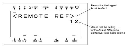
To have the frequency command displayed as the motor speed, load shaft speed, or speed (%), set function code E48 (speed monitor selection) to 3, 4, or 7, respectively, as shown in Table 3.5 Monitored Items.
