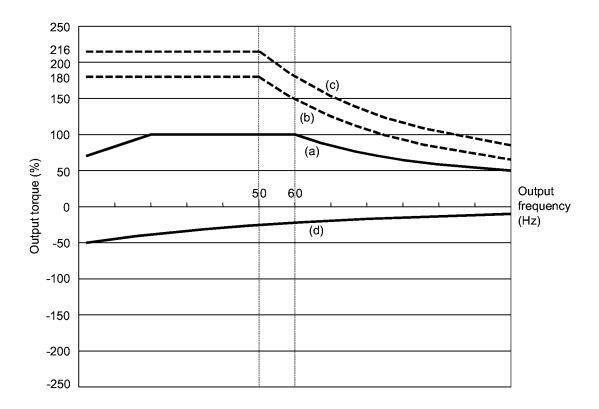
Figure 7.2 Output Torque Characteristics (Base frequency: 60 Hz)
