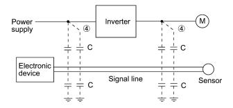
Figure A.5 Electrostatic Induction Noise
