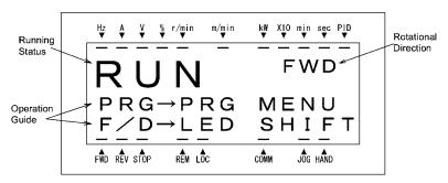
Figure 3.3 Display of Running Status
