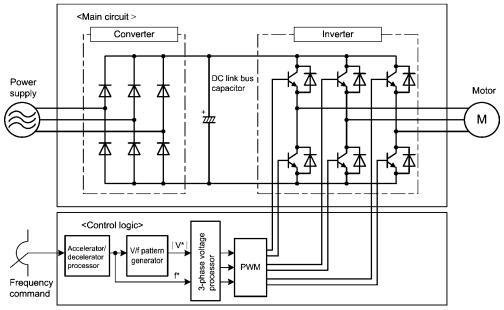
Figure 1.4 Schematic Block Diagram of FRENIC-Eco
