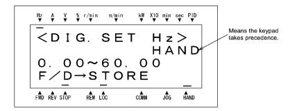
Figure 3.6 Setting the Frequency Command in Local Mode
