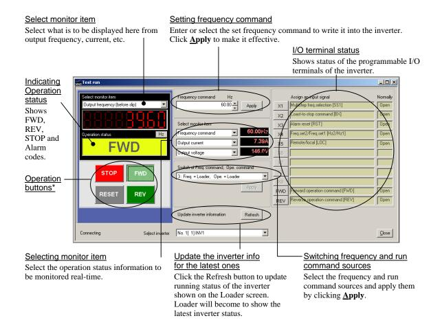
\* Refer to the table shown below for details of the operation buttons. The indented appearance of the **FWD** button as shown in the figure above indicates that it is active for running the motor forward, while that of the REV button is same for running reverse.
