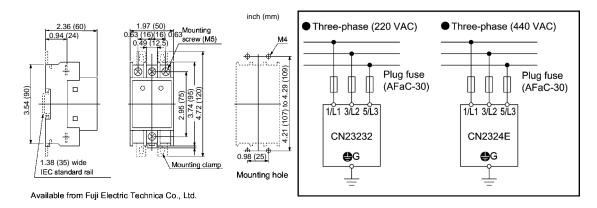
Figure 6.4 Arrester Dimensions and Application Examples
