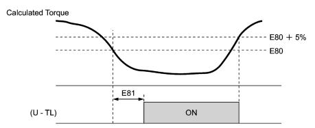
The detection level is set so that 100% corresponds to the rated torque of the motor.
