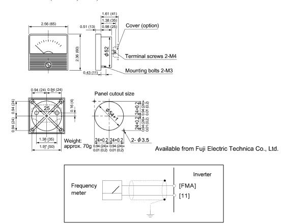
Figure 6.14 Frequency Meter Dimensions and Application Example
