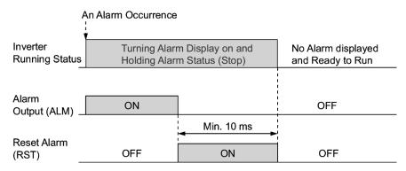
■ Enable external alarm trip -- (THR) (Function code data = 9)
