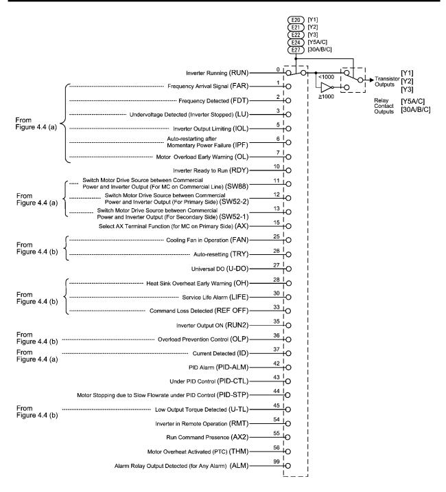
Note: Numerals shown on tap-offs of switches of E20, E21, E22, E24 and E27 are the function code data expressed in the normal (active ON) logic system.
