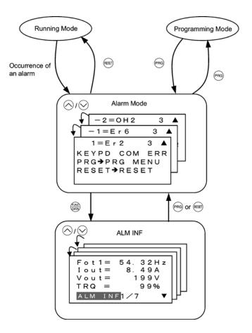
Figure 3.33 Menu Transition in/from Alarm Mode
