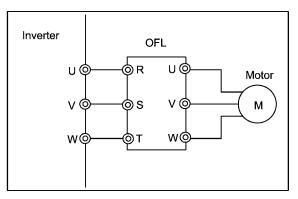
Figure 6.9 External View of OFL and Application Example
