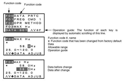
Figure 3.11 Screen for Changing Function Code Data
