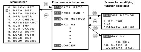
Figure 3.10 Screen Transition for Data Setting Menu
