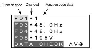
Figure 3.13 LCD Screen Listing Function Codes
