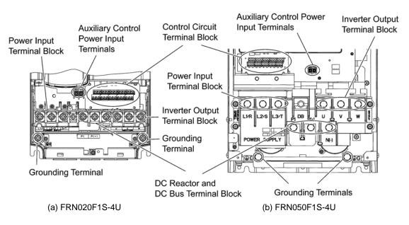
Figure 2.3 Enlarged View of the Terminal Blocks
