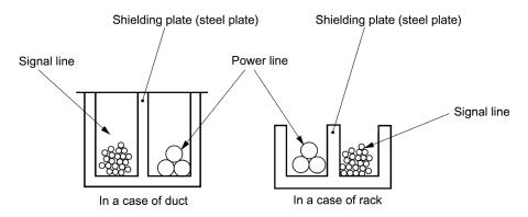
Figure A.7 Separate Wiring
