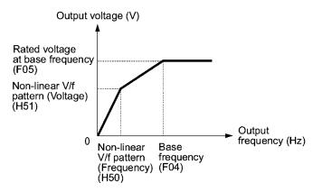
■ V/f Pattern with Non-linear Point above the Base Frequency
