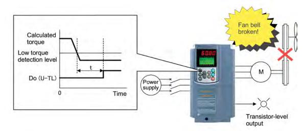
Refer to function codes E20 to E22, E24, E27, E80 and E81 in Section 9.2.2 "E codes."
