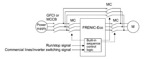
Refer to function codes E01 to E05 in Section 9.2.2 "E codes" and J22 in Section 9.2.6 "J codes."
