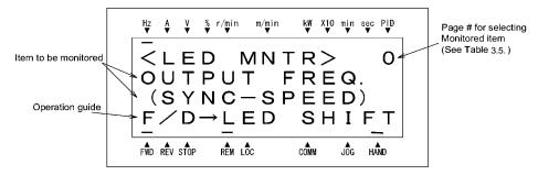
Figure 3.8 Selecting Items to be Monitored on LED Monitor
