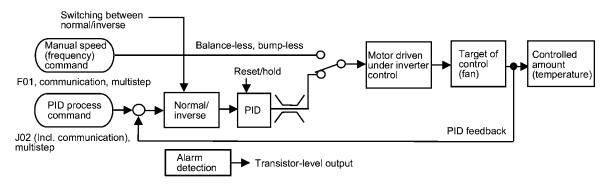
Refer to the PID Frequency Command Generator in Section 4.8, function codes E01 to E05, E20 to E22, E24, and E27 in Section 9.2.2 "E codes," and J01 to J06, J10 to J13, and J15 to J19 in Section 9.2.6 "J codes."
