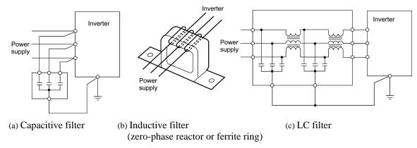
Figure A.10 Various Filters and their Connection
