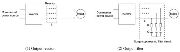
Figure C.3 Method to Suppress Surge Voltage
