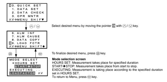
Figure 3.25 Menu Transition for Selecting Measurement Mode
