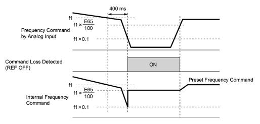
In the diagram above, f1 is the level of the analog frequency command sampled at any given time. The sampling is repeated at regular intervals to continually monitor the wiring connection of the analog frequency command.
