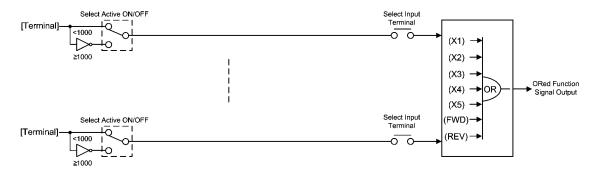
Figure 4.3 (b) Block Diagram of Digital Control Input Block (Only for terminals)
