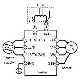
Figure 6.7 Applying a DC Reactor (DCR)
