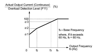
Cooling Characteristics of Motor Equipped with a Shaft-driven Cooling Fan
