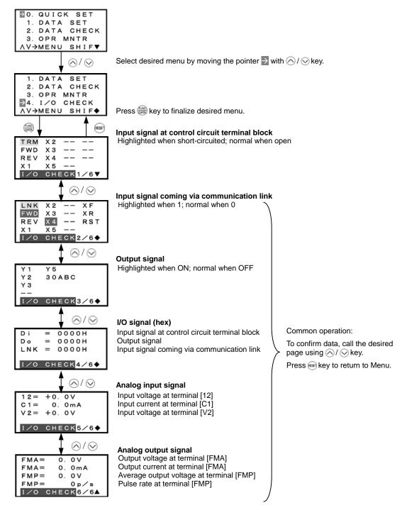
Figure 3.15 Menu Transition for "I/O CHECK"
