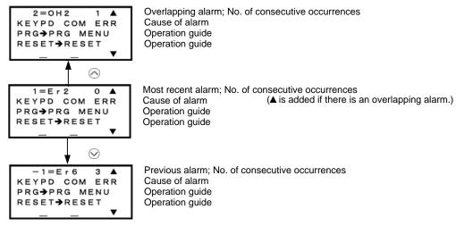
Figure 3.32 Switching of Display of Overlapping Alarm History
