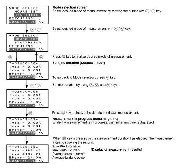
Figure 3.26 Menu Transition for "LOAD FCTR" (hours set mode)
