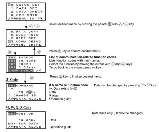
Figure 3.29 Menu Transition for Communication Debugging
