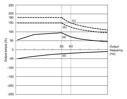
Figure 7.1 Output Torque Characteristics (Base frequency: 50 Hz)
