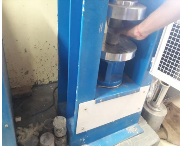
CONCRETE CORE CRUSHING TEST
