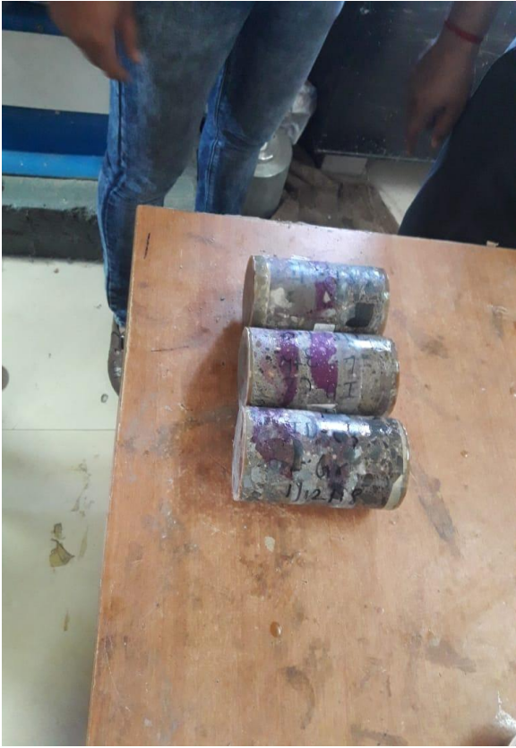
CARBONATION DEPTH TEST ON CORE SAMPLES
