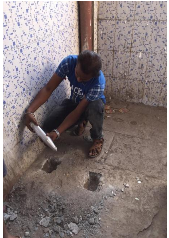
REBOUND HAMMER TESTING ON FLOOR SLAB
