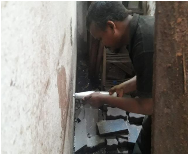
REBOUND HAMMER TEST ON COLUMNS
