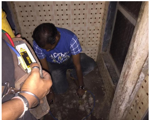
UPV TESTING ON FLOOR SLAB
