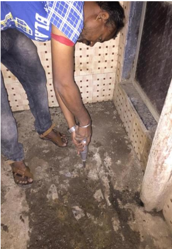
REBOUND HAMMER TEST ON TOP OF SLAB
