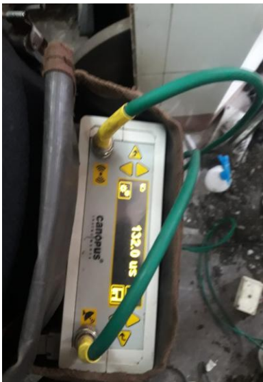
UPV TEST ON COLUMNS
