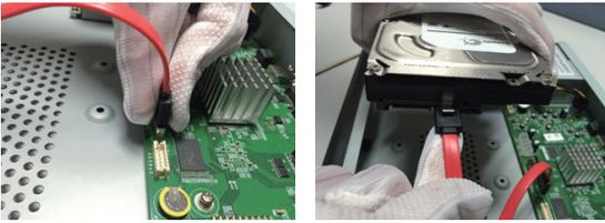
3 Connect one end of the HDD power cable to the SATA interface of the NVR master board, and the other end to the HDD.
