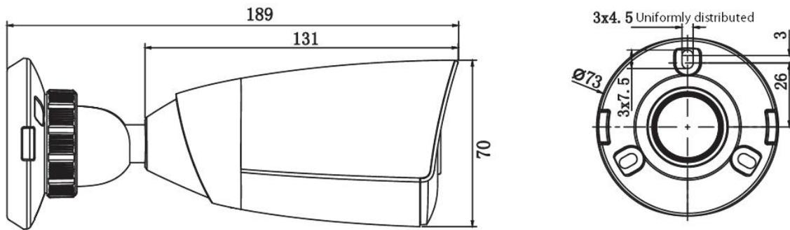
Dimensions of HD Network IR Integrated Machine (MINI)- V2.0
