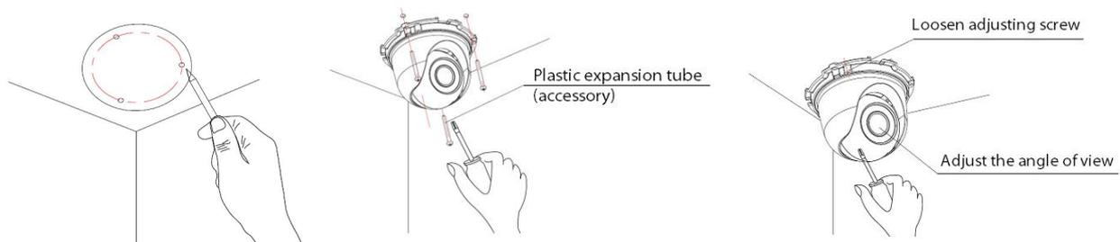
Installation Diagram of HD Network IR Dome Camera (MINI)
