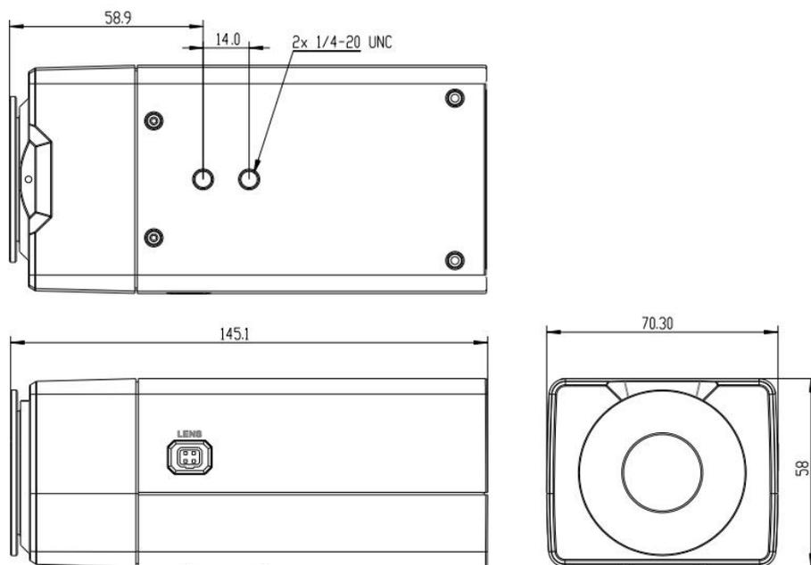
Dimensions of HD Network Gun Camera - V1.0/V2.0
