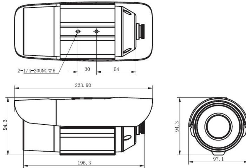
Dimensions of HD Network Zoom IR Gun Camera (without integrated support)
