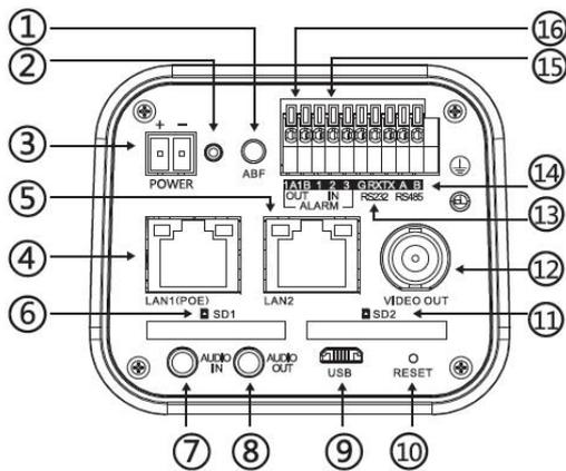
Interface of Type I Network Gun Camera-V3.0
