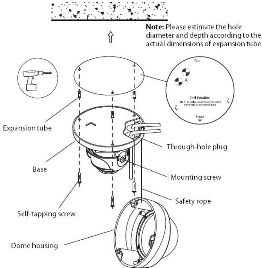
Installation Diagram of HD Network Safe (Non-) IR Dome Camera-V2.0
