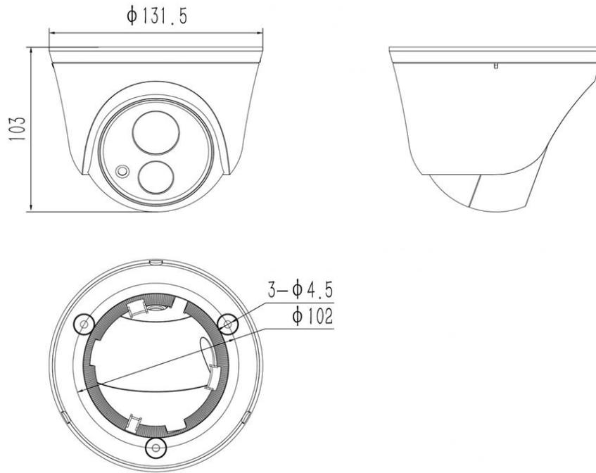
Dimensions of HD Network IR Dome Camera - V4.0
