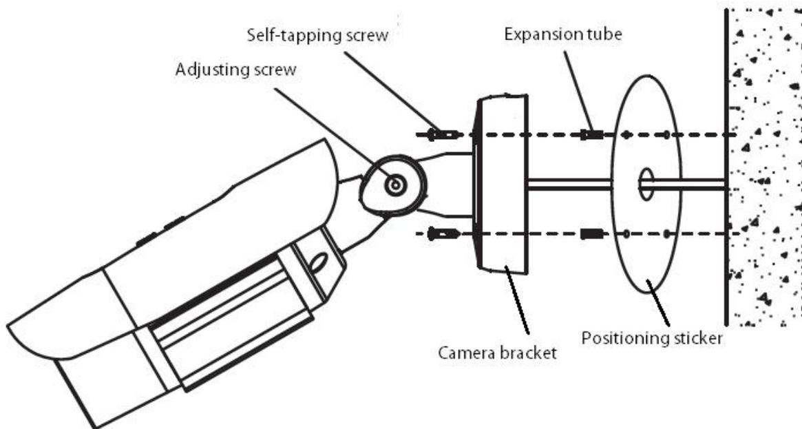
Installation Diagram of HD Network Zoom IR Gun Camera (with integrated bracket)
