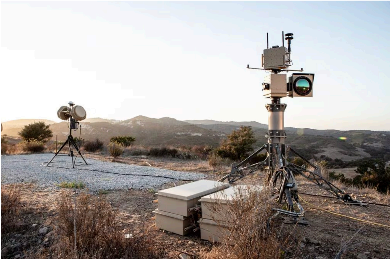
Figure 16 - Anduril autonomous Cruise Missile Defense Sentry Tower ( https://www.defensenews.com/digital-show-dailies/ausa/2020/10/16/anduril-adapts-tech-to-detect-cruise-missiles-in-air-force-demo/ )
