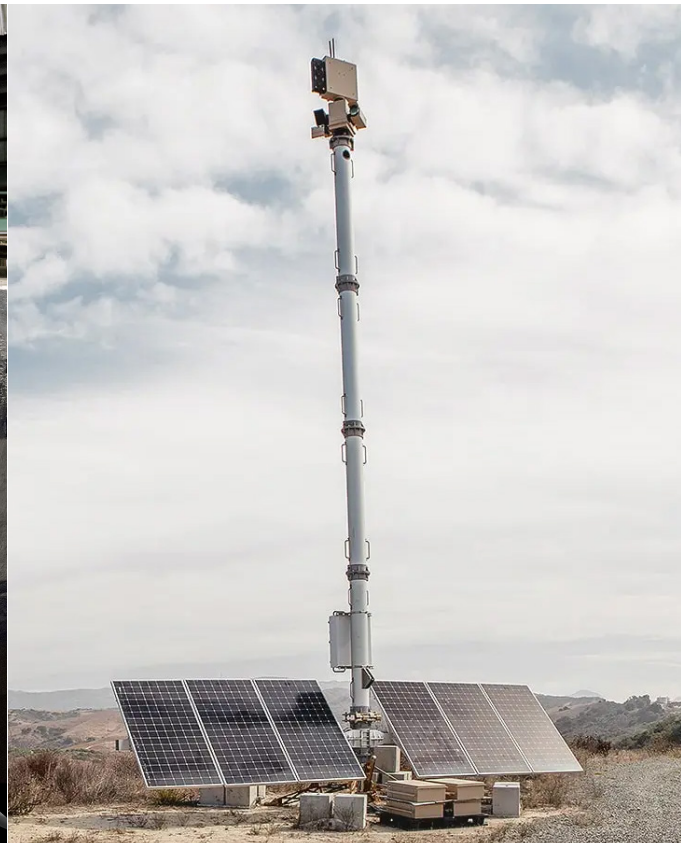
Figure 11 - Autonomous Sentry tower ( https://fedscoop.com/anduril-sentry-towers-cbp/ )
