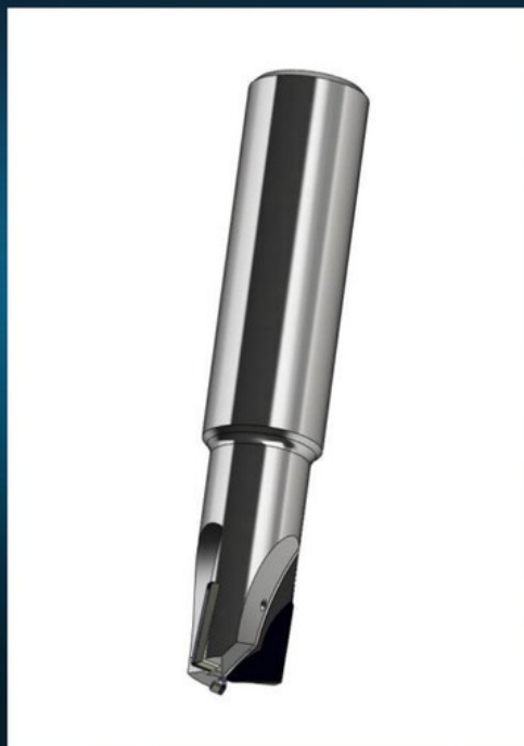
PKD-End mill D12-Z=3 ffor edging of CFK-/GFK- components
