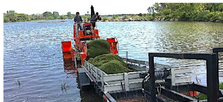
A conveyor off-loads starry stonewort from the harvester to the trailer.
