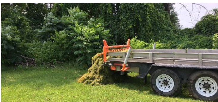
A conveyor on the trailer off-loads starry stonewort at the disposal site.
