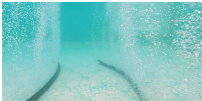
Examples of a pneumatic barrier or bubble curtain created by two sections of bubble tubing.
