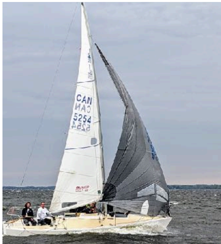
Caught on camera, the moment the headsail on Woodjchuk snagged the lifeline rail and started to rip. D.E.
