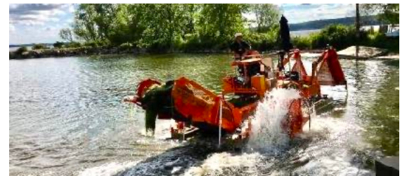
Weeds are stored on board the harvester until they can be discharged to a suitable disposal site on shore. Once cut, it is illegal to allow the weeds, to re-enter the water.
