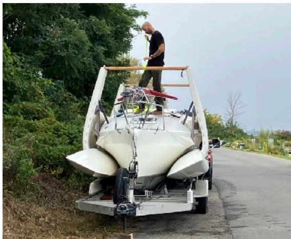
This multi-hull sailboat features a horizontal folding system that allows it to fold for easy trailering. See it opposite E dock. Very cool!!
