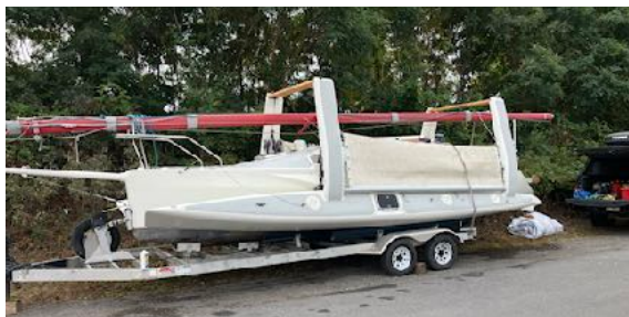
This multi-hull sailboat features a horizontal folding system that allows it to fold for easy trailering. See it opposite E dock. Very cool!!
