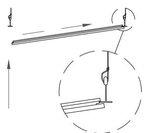
LEVEL THE TILE BY SLIDING FULLY INTO THE SECOND NOTCH, AND BRINGING THE LIP FLUSH WITH THE T-GRID.
