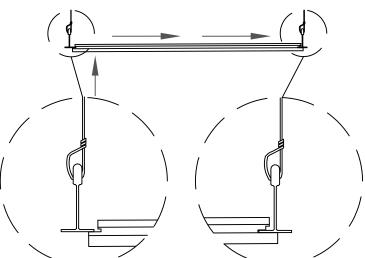
SLIDE THE TILE FULLY INTO THE SIDE WITH THE SINGLE NOTCH, AND ALLOW THE ADJACENT END TO REST ON THE FIRST NOTCH.
