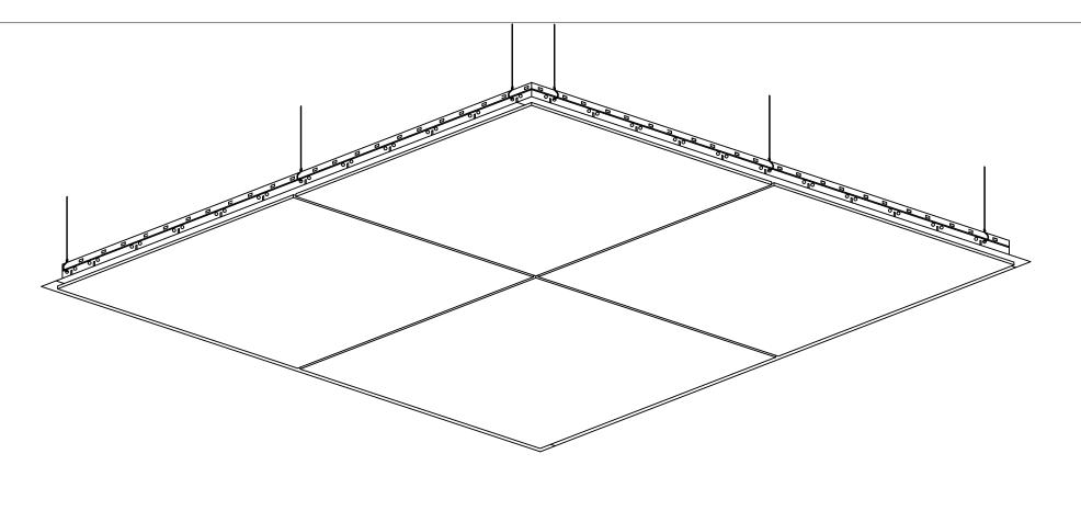
LIFT TILE AT AN ANGLE THROUGH T-GRID OPENING, AND SLIDE INTO THE FIRST NOTCH.
