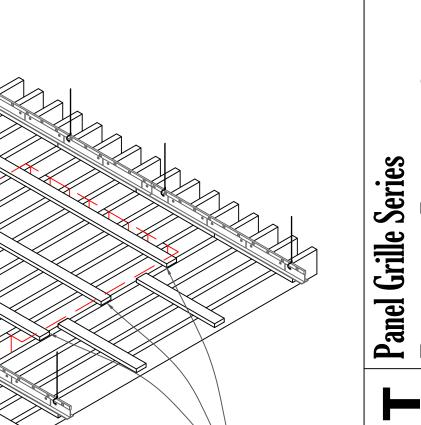
PANEL GRILLE SECTIONS ARE ATTACHED USING (3) BACKER STRIPS PER 24" OPENING. NOTE: BACKERS SHOULD EXCEED ACCESS PANEL OPENING BY (1) BLADE ON EACH SIDE FOR SUPPORT.
