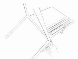
Step 1:Lay the back section of the chair on a table and use the two 3/8" socket head screws to lightly screw in both metal legs
