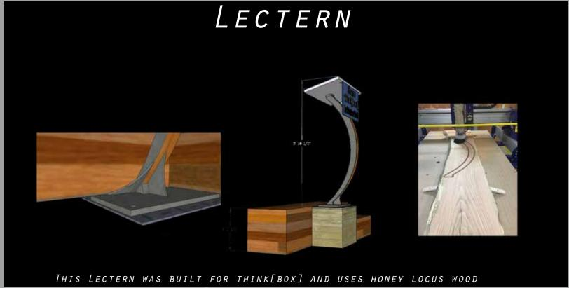
WITH HOT ROLLED STEEL. THE STEEL WAS CUT USING A WATER-JET AND THE WOOD WAS CUT USING A SHOP-BOT. THESE CNC PROCESSES WERE USED WITH PRECISION IN MIND, AS THE FINAL FIT USES NO HARDWARE. FINISHED IN A BLACKENED PATINA AND WAXED TOPCOAT.
