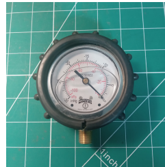
RTM# 4780-01 Composites One# 678113 Vacuum Gauge Liquid Filled 2 1/2" x 1/4" NPT with Rubber Housing Replacement
