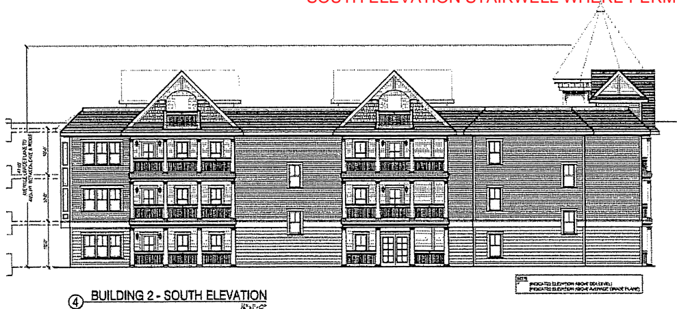
Illustration E.9. — South elevation of Condominium Building Two showing oddly spare single-window fenestration (Sheet A-8).
