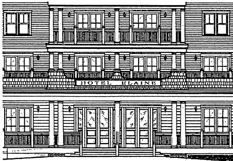
Illustration D.2. — The south elevation (Sheet A-11) showing proposed double set of double ½ doors, with non-conforming single side-light windows to the left and right.
