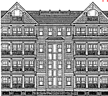
Illustration F.5.a. — Detail of north elevation, Condominium Building One showing paneled areas between windows on projection between balconies (Sheet A-6).
