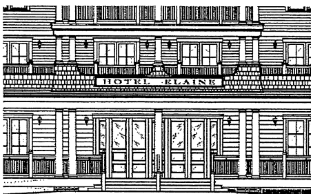
Illustration H.1. — Hotel entrance flanked by double columns with single column bisecting the entry area (Sheet A-11).
