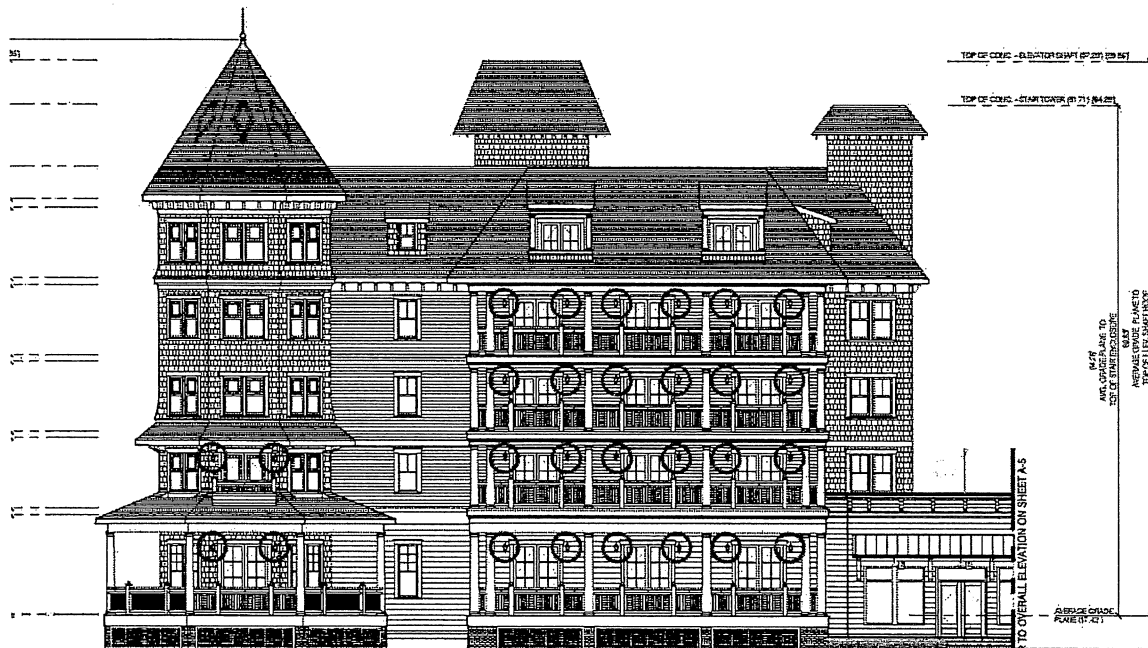
Illustration I.4.b. — East elevation of the Hotel showing twenty-eight (28) proposed lantern fixtures (Sheet A-11).
