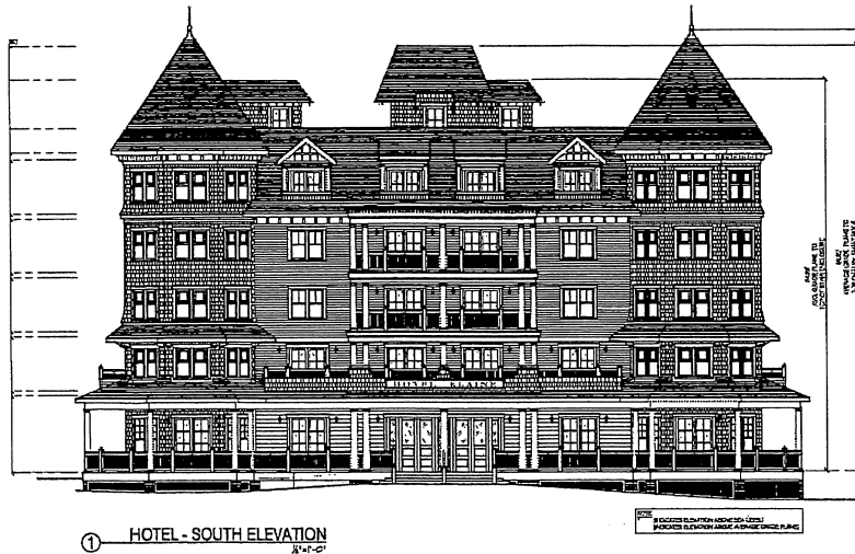
Illustration H.3. — Roof tile patterns showing oversized diamonds and banding (Sheet A-11).
