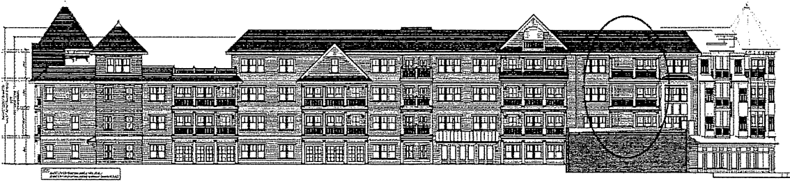
Illustration I.10. — South elevation of Condominium Building One showing balconies with no lighting indicated.
