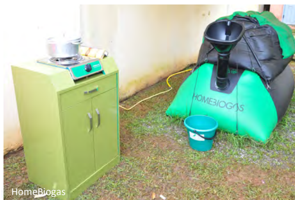
Examples of anaerobic biogas digesters. Top : shows a medium-scale operation. Bottom : shows a small-scale domestic unit.
