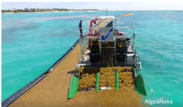
AlgeaNova's sargassum harvesting boat working along the outside of the sargassum barrier.
