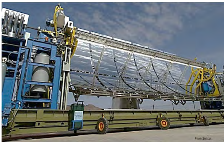
The industrial-sized solar microwave oven (SMO) for valorisation of organic biomass and organic waste
