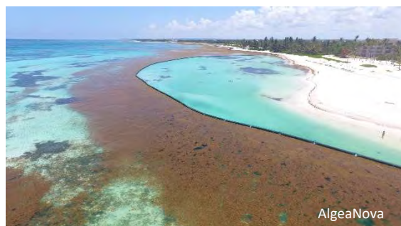
AlgeaNova's floating barrier in Punta Cana holding sargassum off the beach ready for collection
