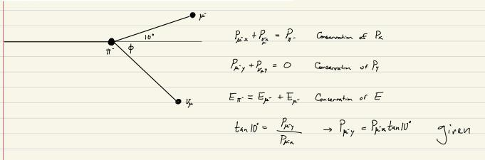
$$E_{\pi} = \sqrt{m_{p}^{2}C^{4} + p^{2}c^{2}} = \sqrt{m_{\mu}^{2}C^{4} + (p_{\mu x}^{2} + p_{\mu y}^{2})c^{2}} + \sqrt{(p_{\mu x}^{2} + p_{\mu y}^{2})c^{2}}$$
