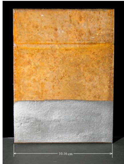
Figure 12 Initial corroded surface of as-received ABS-A specimen prior to cleaning (top) and after bristle blast cleaning (bottom).
