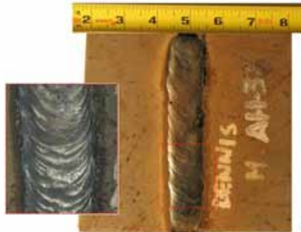
Figure 9 Front weld bead and weld pool segment (inset) of AH-36 welded specimen.
