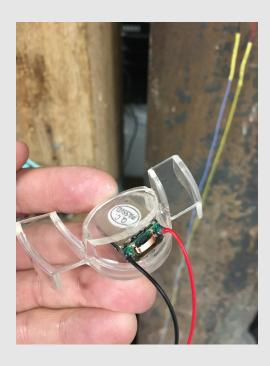
Insert transducer into opening, wires coming out of the open end.
