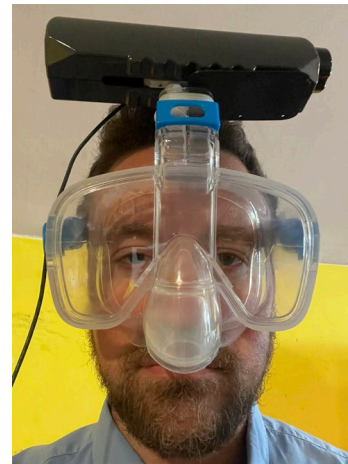
Figure 7. Breath-based Morse Interface (2024). Nose snorkel, 3D printed mount, Jamboxx midi harmonica (in/out breath sensor).
