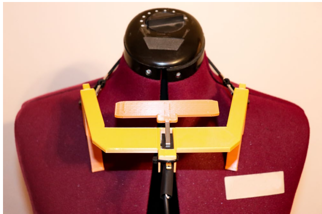
Figure 2. One-button Chin Interface (2024). Microswitch mounted in a 3D printed frame, neck cord, quarter inch output.
