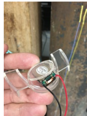
Figure 1. Mantra Mouthguard (2018). Audio transducer (bone conductor) in an LED mouthpiece with LED removed.
