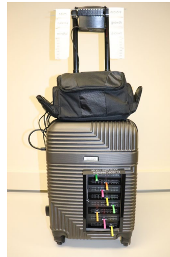
Figure 6. Carry-on for Consciousness (2024). 20" hardshell carryon luggage bag with a 5" x 9" rectangular section cut from the front, a Behringer X-Touch Compact, an Arduino micro, ten microswitches in a 3D printed frame attached to the carryon handle, a Windows laptop running Max for Live, Ableton Live 12, Bome Midi Translator Pro, and two Roland TM-1s to receive the signals from the sensors.
