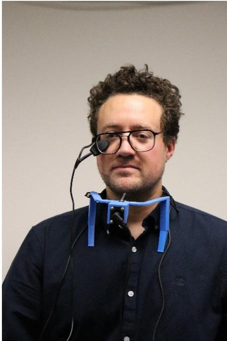
**Figure 4: Eye Blink Switch mounted to glasses. Chin Interface worn around neck is activated by the traveler chewing gum.**
