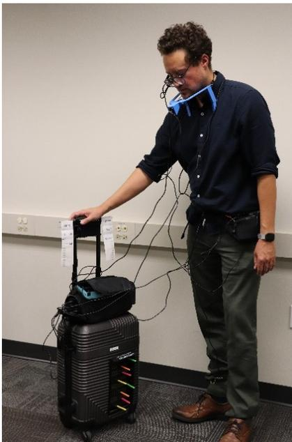
Figure 2: The Carry-on for Consciousness connected to wearable sensors and traveler.
