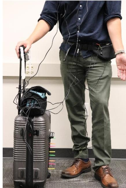
**Figure 5: Fanny Pack holds magnetic reed switch. Magnet attached to Apple Watch band activates switch in fanny pack with each arm swing.**
