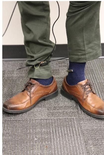
**Figure 6: Step sensors. Magnetic reed switch zip-tied to right leg. Magnets worn on inside and outside of left sock activate switch each step.**
