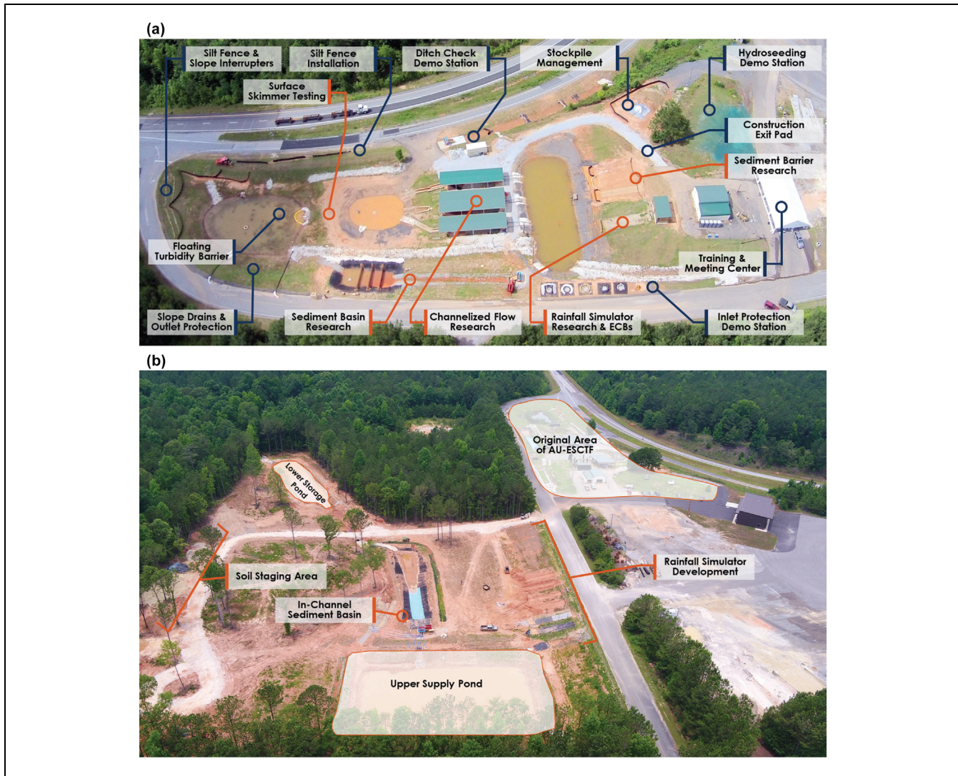
Figure 1. Auburn University erosion and sediment control test facility: (a) before expansion, and (b) post expansion (2021). Note: AU-ESCTF = Auburn University Erosion and Sediment Control Testing Facility; ECB = Erosion Control Blanket.
