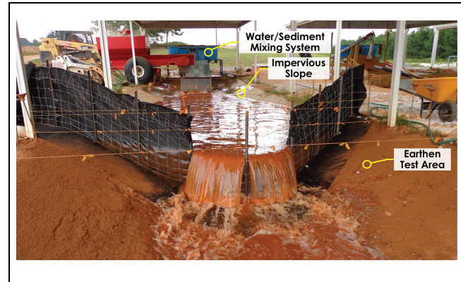
Figure 3. Photo of ditch check (DC) test apparatus.
