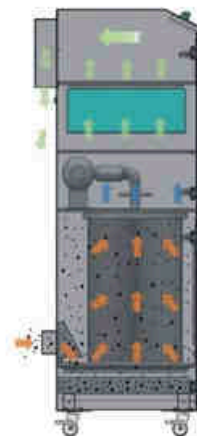
TS-LT-HP-IQ Series purification schematic
