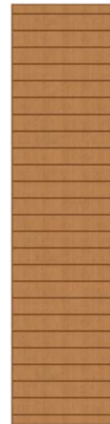
1-1/2" Thick MDF core panel with veneer slat wall with solid banding on 4 sides
