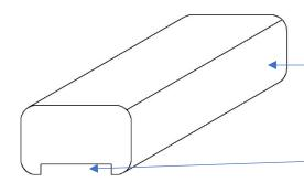
The wood grabber has 2 parts, #1 the top, and #2 the fillet which is underneath. The fillet, fills in between the posts, giving strength to the top.
