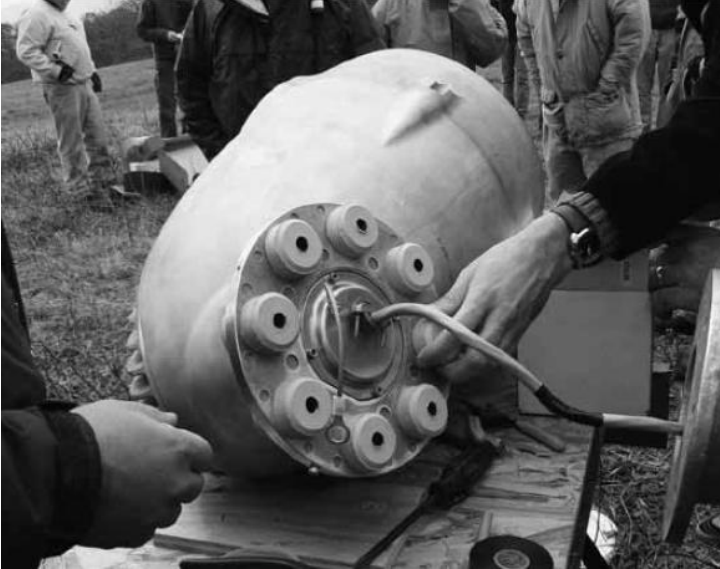
Figure 8 Placing vibration isolators
