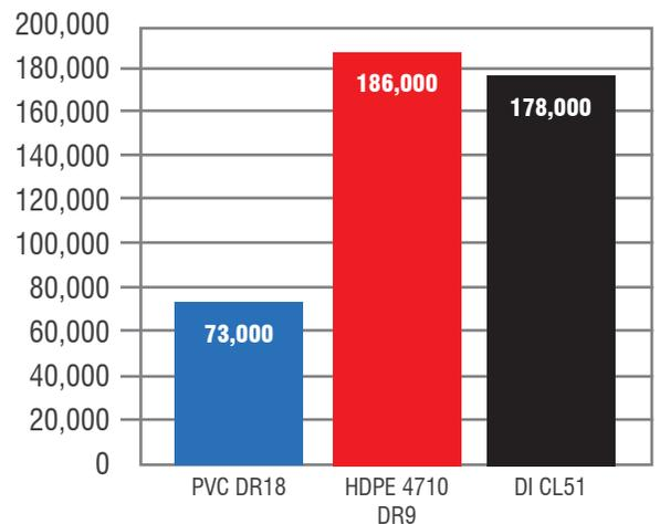
**FIGURE 10.4 : COMPARISON OF AVERAGE ANNUAL 100-YEAR PUMPING ENERGY COSTS PER 1,000 MILES OF PIPE BASED ON 0.4 FPS VELOCITY**
