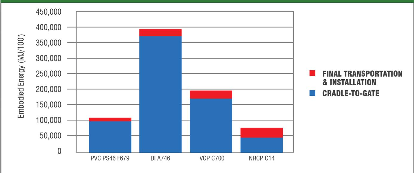
**FIGURE 12.9 : TOTAL 100-YEAR EMBODIED ENERGY FOR 24" PVC PS46 SOLID-WALL & PROFILE-WALL EQUIVALENT GRAVITY PIPES**
