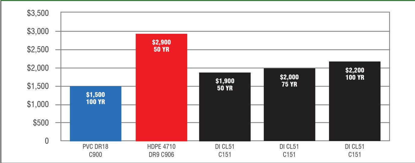
**FIGURE A.22 : 24" PVC DR25 EQUIVALENT PIPES TOTAL 100-YEAR PUMPING COSTS USING DIFFERING PIPE LIVES (\$/100'/100 YRS.)**
