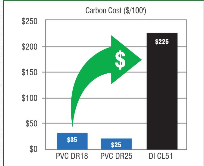
**TABLE 10.1 : COMPARISON OF MONETIZED CARBON OUTPUT OF PIPE MATERIALS PER 100 FEET OF 8" PIPE**
