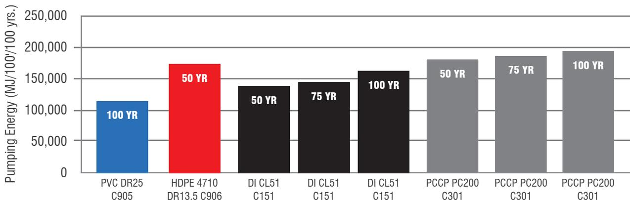
**FIGURE A.21 : 8" PVC DR18 EQUIVALENT PIPES TOTAL 100-YEAR PUMPING COSTS USING DIFFERING PIPE LIVES (\$/100'/100 YRS.)**
