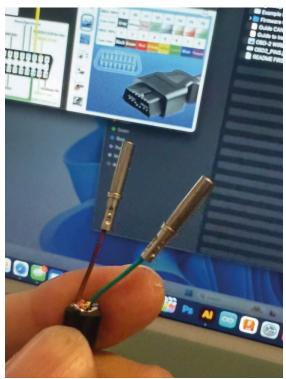
5. And then insert the terminals into the connector like this
